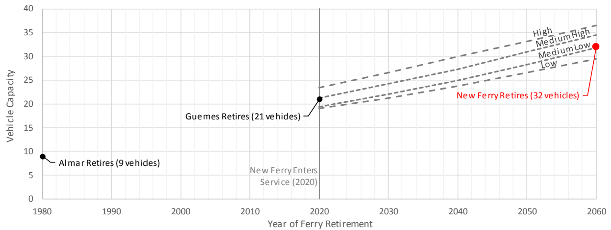
Figure 2 Vehicle capacity history and forecast with four growth trends (medium-low chosen)
